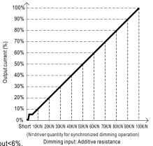
Note: 1. Min. dimming level is about 6% and the output current is not defined when 0% < Iout < 6%.
