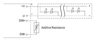
"DO NOT connect "DIM- to -V"
