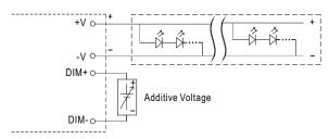
"DO NOT connect "DIM- to -V"
