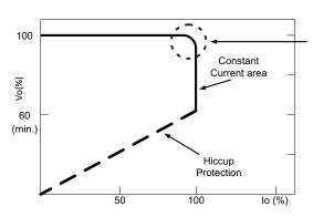
Typical LED power supply I-V curve
