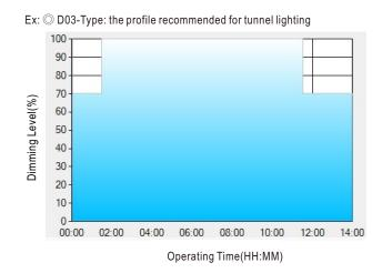
Set up for D03-Type in Smart timer dimming software program:
