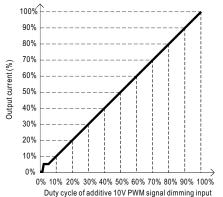
90% 80% Output current (%) 60% 50% 40% 30% 20% 10% Short 10K/N 20K/N 30K/N 40K/N 50K/N 60K/N 70K/N 80K/N 90K/N 100K/N  $(N \hbox{=} driver \ quantity \ for \ synchronized \ dimming \ operation)$
