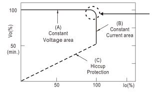
Typical output current normalized by rated current (%)
