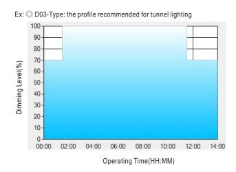
Set up for D03-Type in Smart timer dimming software program:
