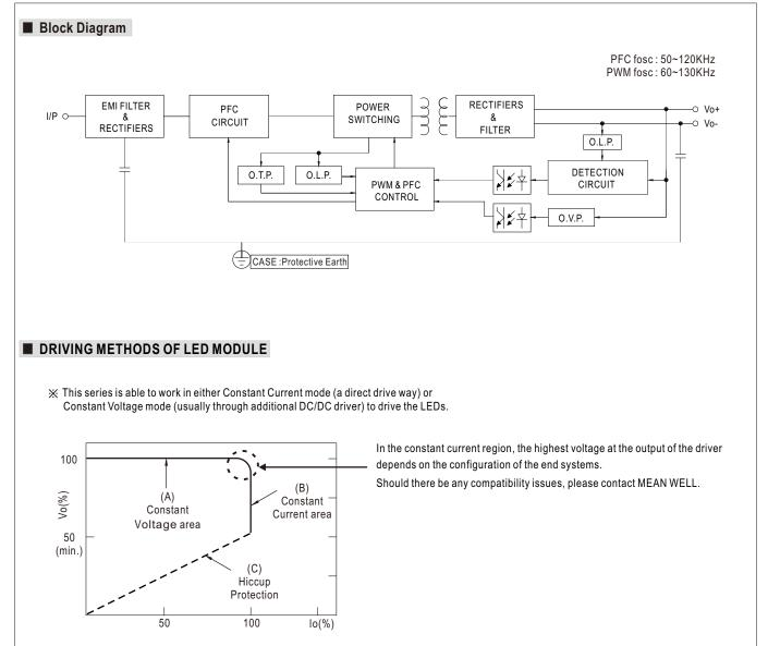
Typical output current normalized by rated current (%)
