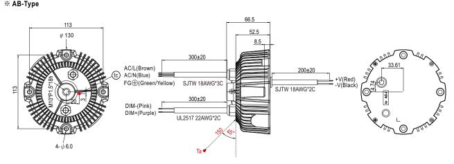
• (tc) : Max. Case Temperature.(case temperature measured point)
