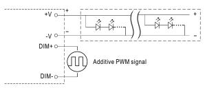
"DO NOT connect "DIM- to -V"
