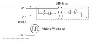
"DO NOT connect "DIM- to -V"
