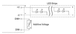
"DO NOT connect "DIM- to -V"
