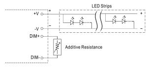
"DO NOT connect "DIM- to -V"
