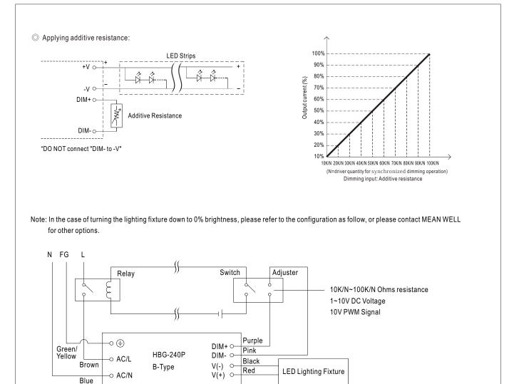
Using a switch and relay can turn ON/OFF the lighting fixture.
