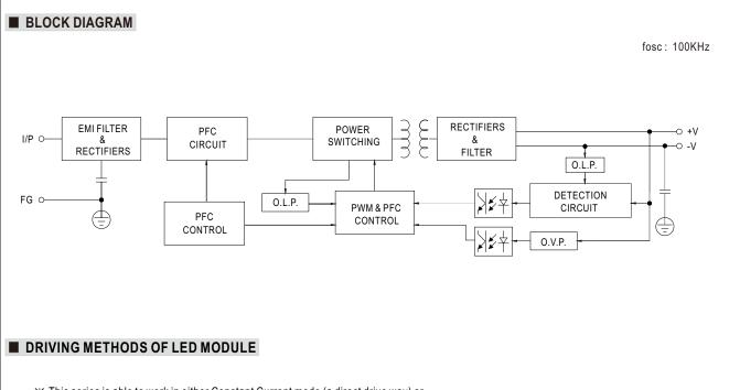
This series is able to work in either Constant Current mode (a direct drive way) or Constant Voltage mode (usually through additional DC/DC driver) to drive the LEDs.
