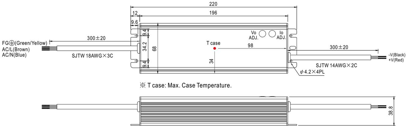
※ IP65 rated. Output voltage and constant current level can be adjusted through internal potentiometer.
