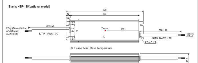
※IP68 rated. Cable for I/O connection.
