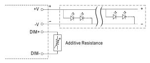
"DO NOT connect "DIM- to -V"
