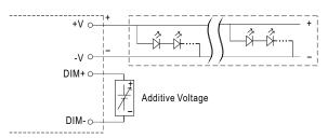
"DO NOT connect "DIM- to -V"
