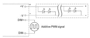
"DO NOT connect "DIM- to -V"
