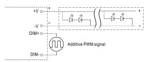
"DO NOT connect "DIM- to -V"
