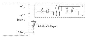
"DO NOT connect "DIM- to -V"
