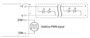
"DO NOT connect "DIM- to -V"
