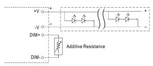
"DO NOT connect "DIM- to -V"
