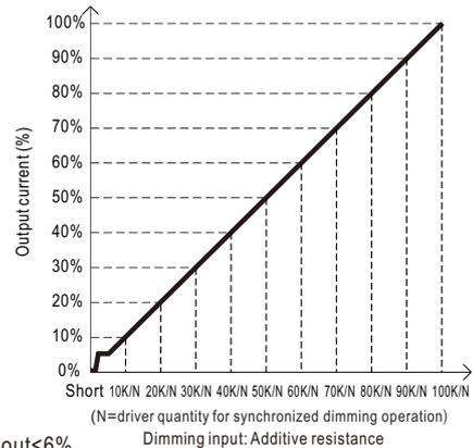
Note : 1. Min. dimming level is about 6% and the output current is not defined when 0% < I<sub>out</sub> < 6%.
