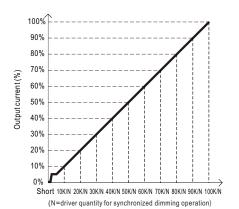
Dimming input: Additive resistance Note: 1. Min. dimming level is about 6% and the output current is not defined when 0%< Iout<6% 2. The output current could drop down to 0% when dimming input is about 0kΩ or 0Vdc, or 10V PWM signal with 0% duty cycle.
