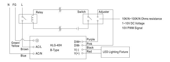
Using a switch and relay can turn ON/OFF the lighting fixture.
