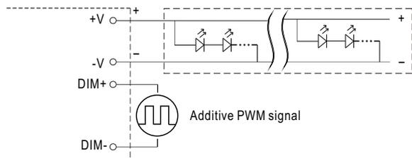
"DO NOT connect "DIM- to -V"
