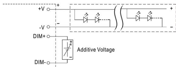
"DO NOT connect "DIM- to -V"
