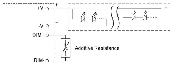
"DO NOT connect "DIM- to -V"
