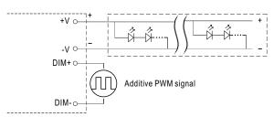
"DO NOT connect "DIM- to -V"
