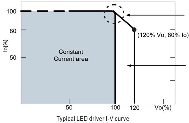
In the constant current region, the highest voltage at the output of the driver depends on the configuration of the end systems.
