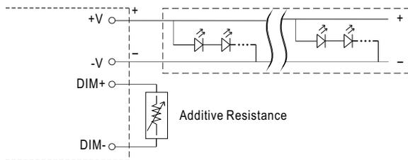
"DO NOT connect "DIM- to -V"
