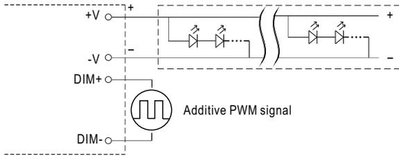
"DO NOT connect "DIM- to -V"
