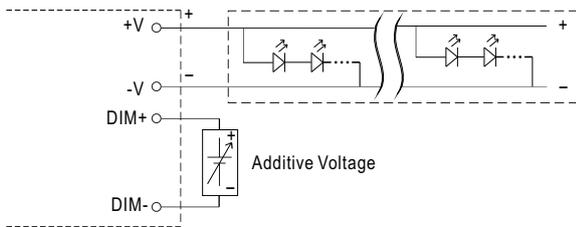
"DO NOT connect "DIM- to -V"
