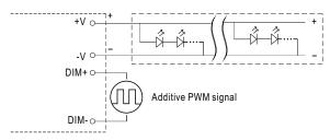
"DO NOT connect "DIM- to -V"
