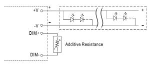
"DO NOT connect "DIM- to -V"
