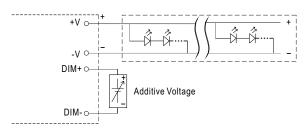
"DO NOT connect "DIM- to -V"
