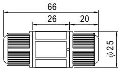
CJ04-1 suitable for 14AWG~16AWG
