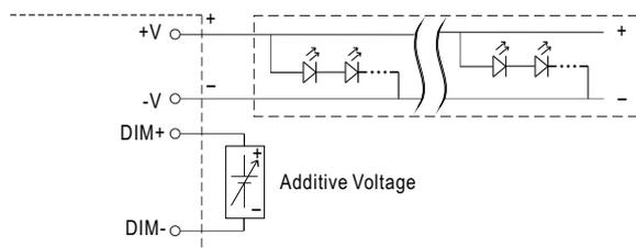
"DO NOT connect "DIM- to -V"
