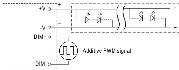
"DO NOT connect "DIM- to -V"
