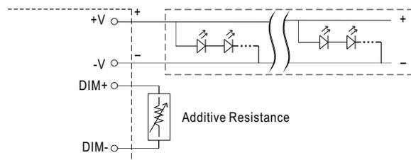
"DO NOT connect "DIM- to -V"
