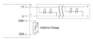
"DO NOT connect "DIM- to -V"
