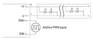
"DO NOT connect "DIM- to -V"
