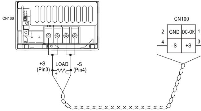
Fig 2.1 Sense lines should be twisted in pairs
