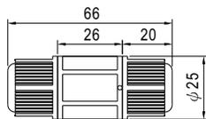
CJ04-1 suitable for 14AWG~16AWG
