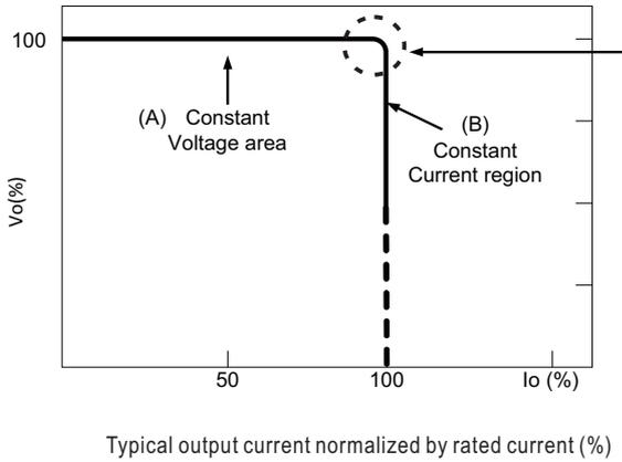
In the constant current region, the highest voltage at the output of the driver depends on the configuration of the end systems.
