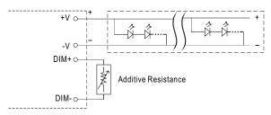
"DO NOT connect "DIM- to -V"
