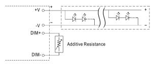
"DO NOT connect "DIM- to -V"
