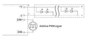
"DO NOT connect "DIM- to -V"
