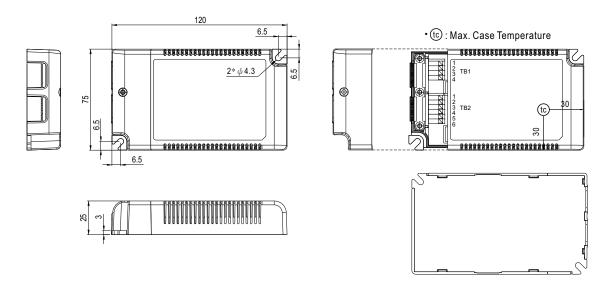
NOTE: Please use wires with a cross section of 0.75~1.5mm $^2$  for TB1 and wires with a cross section of 0.5~1.5mm $^2$  for TB2.
