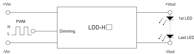
Fig-1 12VDC input, 1~3 LEDs (Vf=3V)
