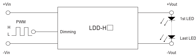
Fig-1 12VDC input, 1~3 LEDs (Vf=3V)
