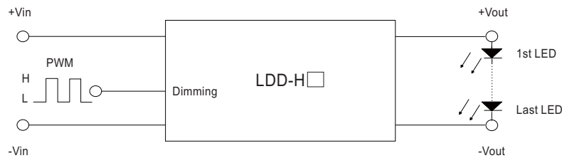
Fig-1 12VDC input, 1~3 LEDs (Vf=3V)
