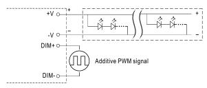
"DO NOT connect "DIM- to -V"
