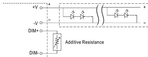
"DO NOT connect "DIM- to -V"
