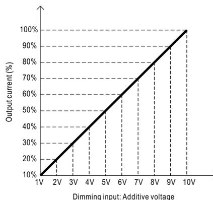
◎ Applying additive 10V PWM signal (frequency range 100Hz ~ 3KHz):
