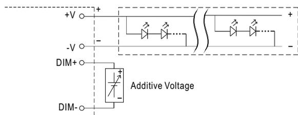
"DO NOT connect "DIM- to -V"
