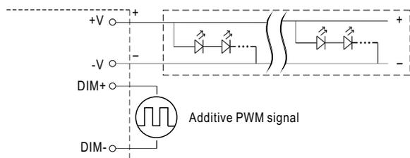
"DO NOT connect "DIM- to -V"
