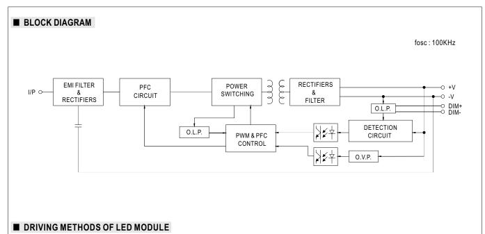
% This series works in constant current mode to directly drive the LEDs.
