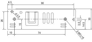
Case No.239A Unit:mm Tolerance:±1
