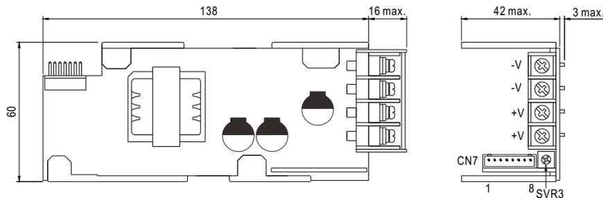
Output Connector(CN7) : JST B8B-XH or equivalent
