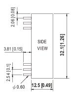
NOTE: Pin tolerance ±0.5mm
