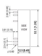
NOTE: Pin tolerance ±0.5mm
