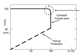
Typical LED power supply I-V curve
