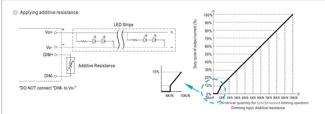
Note: 1. Min. duty cycle of output current is about 6% and the output current is not defined when 0%< Iout<6%.
