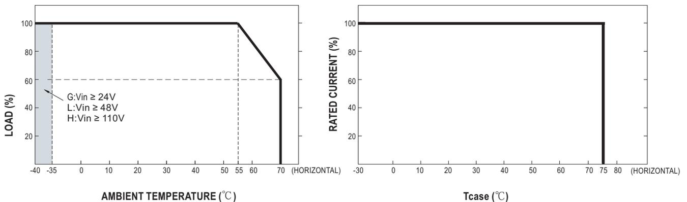
Suitable installation methods are shown as below. Since RSD-30 is a semi-potted model, its thermal performances for the following installation methods are similar and share the same derating curve.
