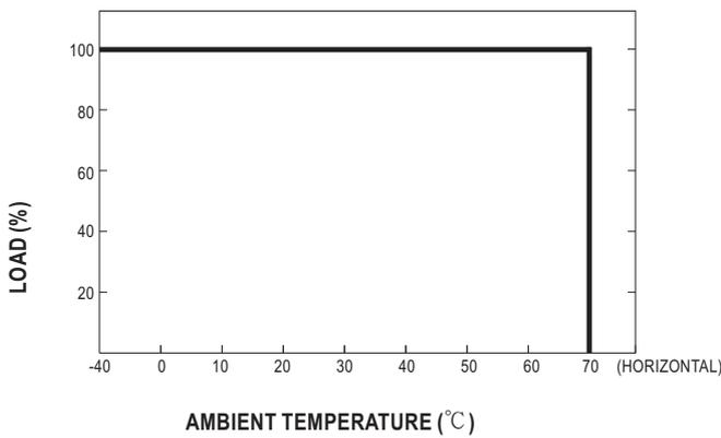
Suitable installation methods are shown as below. Since RSD-30 is a semi-potted model, its thermal performances for the following installation methods are similar and share the same derating curve.
