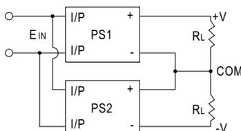
2. Increase the output voltage (current does not change). Because RSD-30 series have no reverse blocking diode in the unit, you should add an external blocking diode to prevent the damage of every unit while starting up. The voltage rating of the external diode should be larger than  $V1+V2$  (as shown as below).
