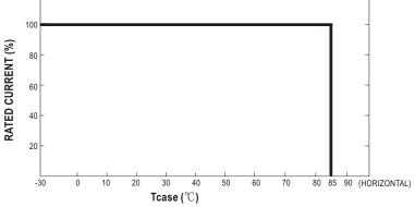
Suitable installation methods are shown as below. Since RSD-500 is a semi-potted model, its thermal performances for the following installation methods are similar and share the same derating curve.
