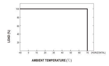
Suitable installation methods are shown as below. Since RSD-500 is a semi-potted model, its thermal performances for the following installation methods are similar and share the same derating curve.
