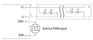
"DO NOT connect "DIM- to -V"
