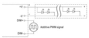
"DO NOT connect "DIM- to -V"
