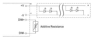
"DO NOT connect "DIM- to -V"
